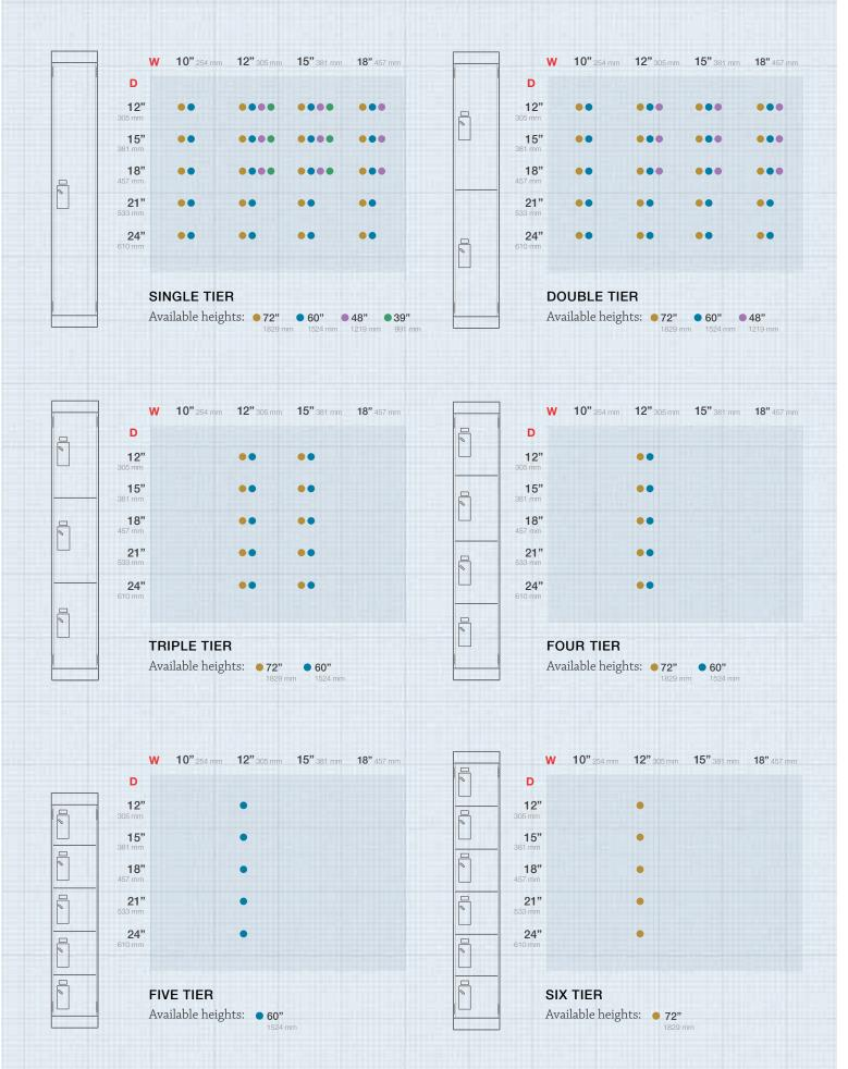
Positive latch is not available for 72" (1829 mm) high six tier or 60" (1524 mm) high five tier lockers.
