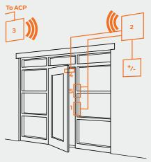
The WRI400 wireless reader interface is a networked access point controller designed to provide wireless connectivity to traditional electronic access control components, including standard Wiegand readers, door position, tamper, and request to exit switches.
