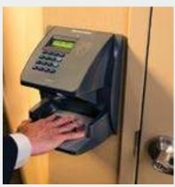
Hand geometry measures the unique size and shape of an individual's hand making it highly reliable and secure. Hand readers provide the best combination of speed and accuracy, making them the easiest biometric to use.
