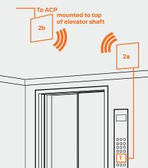
The ECK400 wireless elevator kit is ideal for retrofit applications, it eliminates the need to run traveling cables inside the elevator shaft. The reader is connected to the WRI400 on top of the cab. The WRI400 communicates over 900 MHz to the PIM400 on top of the shaft. The PIM400 is wired back to the ACP for real time monitoring.
