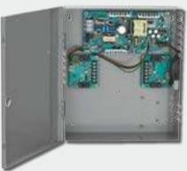
Schlage and Von Duprin power supplies feature a flat mounting design and polarized locking connectors for option boards. This design eliminates the need for racks and side connectors, and provides easier access to the terminal blocks for connection of peripheral devices including strikes, electromagnetic locks and card readers.
