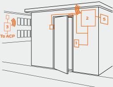
The WRI400 has a communication range of up to 1,000 ft. with clear line of sight. Remote antennas can be used to increase the range when needed. The WRI400 eliminates the need to dig a trench to the storage shed, saving time and money associated with equipment rental and running wires under ground.
