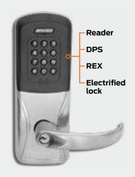
The AD Series combines the electrified lock, reader, door position and REX switches together into one device for simplified installation and connection to the access control panel. Hardwired and wireless options are available.
